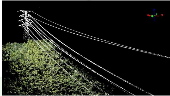
Powerline laser point cloud with RGB value
